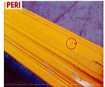
PERI MULTIPROP MP250, 350 & 480 have locating 'notches' on the yellow casing (the MP120 & 625 do not); the counterfeit version does not.
