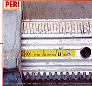
The measuring tape inside the PERI MULTIPROP has 'PERI' on it. There is one rivet at each end of the tape, whereas the counterfeit version has rivets along its entire length.
